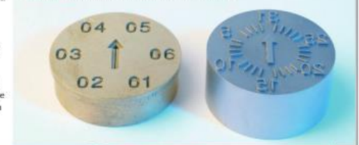
<< Figure 5: Mould insert and PEM electrode. >>
