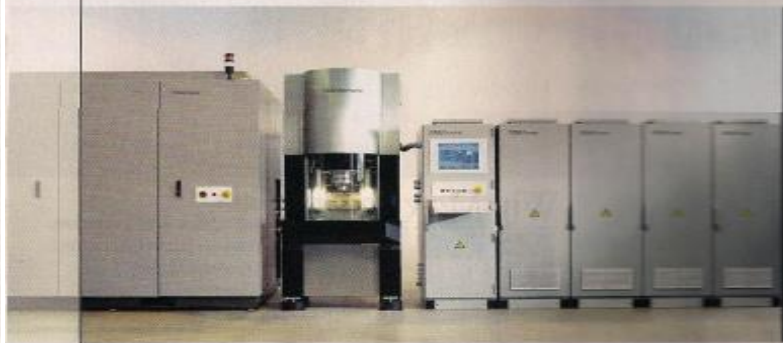
A PEM machining center consists of four primary components (the machine itself, power supply, control and electrolyte systems) that can be arranged in a variety of configurations to suit specific facility layouts.
