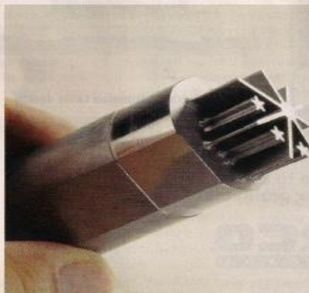
Once produced as four separate tools via wire EDM, the star- and sun-shaped features shown here are now part of a single precision punch produced with PEM. Note the undercut around the entire geometry.
